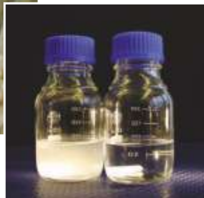
Struvite (Magnesium-Ammonium-Phosphate) in combination with sludge/polymer deposits.
