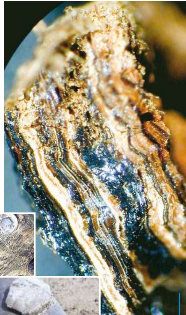
Microscope view of crystals layers (Struvite) [Mg(NH_4)(PO_4) \cdot 6H_2O]
